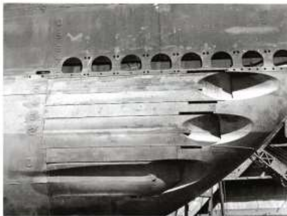
Caption: Tullibee's forward torpedo tubes, this view showing the starboard bow tube with the shutters in the closed position. Note the draft marks welded onto the hull, painted the same color as the surrounding hull, Pearl Harbor Navy Yard, 24 May 1943. (U.S. Navy Bureau of Ships Photograph, 19-LCM Box 540, National Archives and Records Administration, Still Pictures Division, College Park, Md.)
